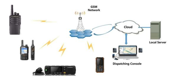
Voice communication is transmitted digitally from the radio terminal to your nearest GSM tower, from the tower it utilizes the IP backhaul from the tower to our locally hosted servers, which in return translates voice into secure crystal-clear audio being delivered to and from the Neco-Guardian devices.
